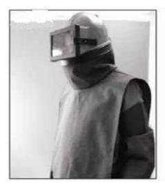
Fit helmet comfortably on head, tighten cape
